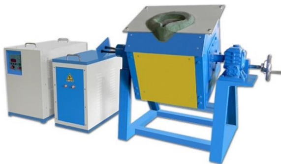
1-rasm. Induksion tok yordamida metall eritish jihozi JLZ-35kW 10 kg.
