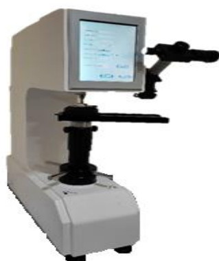
3-rasm. THBRV-187.5DX Universal qattiqlikni o'lchash mashinasi
